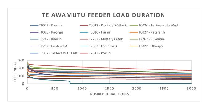
The Company then makes predictions of when its feeders will become capacity constrained, voltage constrained or security constrained in accordance with the established criteria and a growth rate of 3.0% per year.
